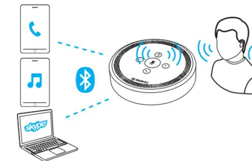
**Bluetooth Pairing Mode** M1 enters Bluetooth pairing mode automatically for the first use. Press and hold Bluetooth button for 3 seconds to switch Bluetooth device. Bluetooth light flashes fast.
