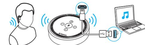
**Entering USB mode:** Connect M1 to your device by using a USB cable and USB light turns solid orange.
